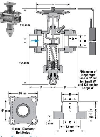
**Specifications** – Element Size No. 63, Small Capacity No. 7 Large Capacity – Gasket Joint, Standard Tubing Length 3 Meters® Flange Ring Size – 2-3/4" OD x 2-3/16" ID.
