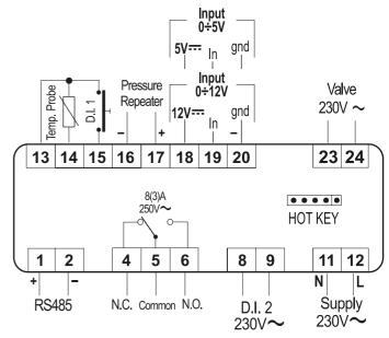
**24-110Vac Models:** Power supply, high voltage digital input and valve output are respectively 24Vac or 110Vac.
