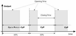
With opening percentage we mean percentage of cycle period where valve is open. For example, if CyP=6s and we say: "The valve opening percentage is 50%"; we mean the valve is opened for 3s during cycle period.
