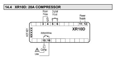
24Vac/dc supply: connect to the terminals 11 and 12. 120Vac supply: connect to the terminals 11 and 12. 230Vac supply: connect to the terminals 11 and 12.
